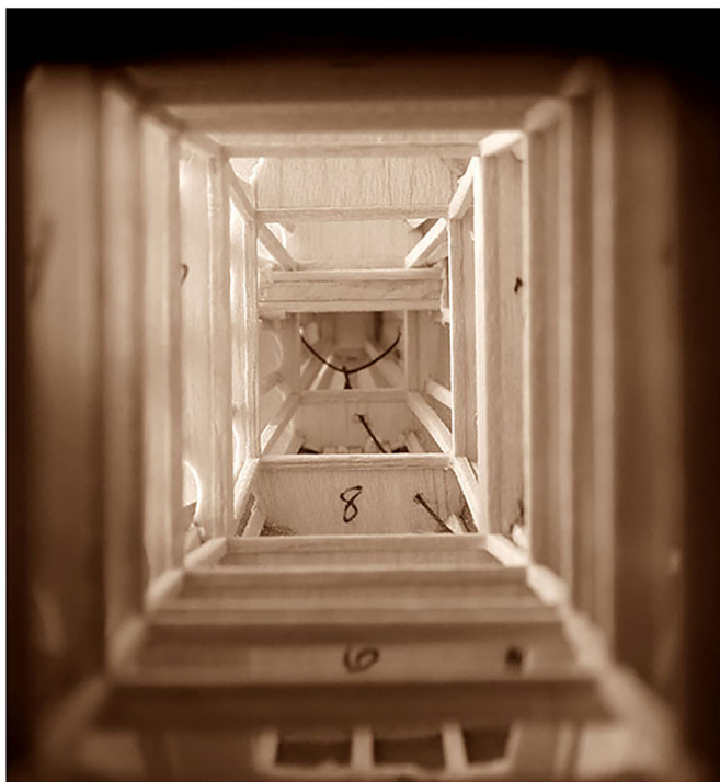
Figure 3, inside of the model with DT line running through formers, far away from the flailing rubber motor.
