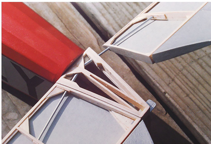
Figure 6, Gadfly stab with aluminum DT pivots installed and plywood stab stops visible.
