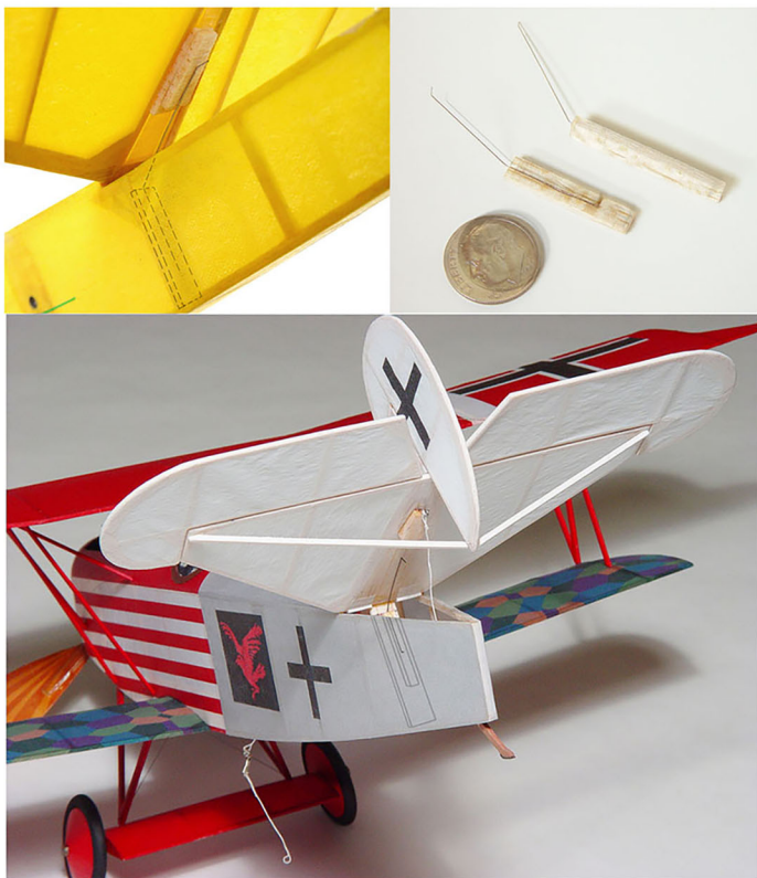
Figure 11, Top Left: Cassna stab in DT configuration held in position by small guitar wire spring. Right: guitar wire spring glued to balsa base and ready for installation in fuselage. Bottom: Fokker DVII wit stab DTed and spring hilding the stab up.
